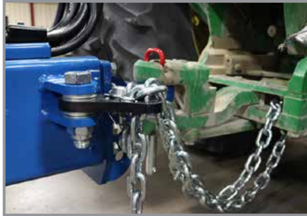
Drawbar and safety chain connection
