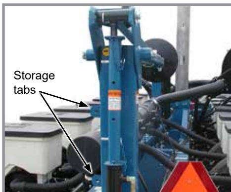
Row marker lockup installed
