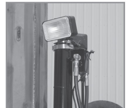
Auxiliary work lights
