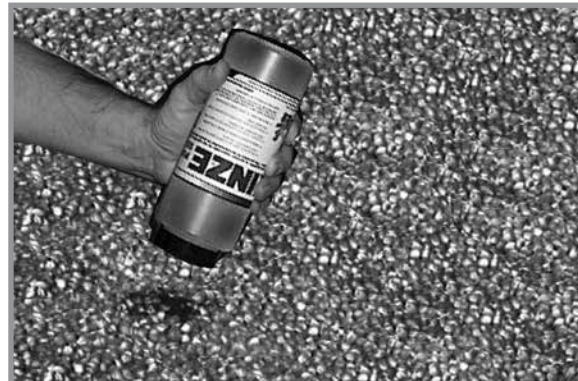
Adding graphite bulk fill hopper
