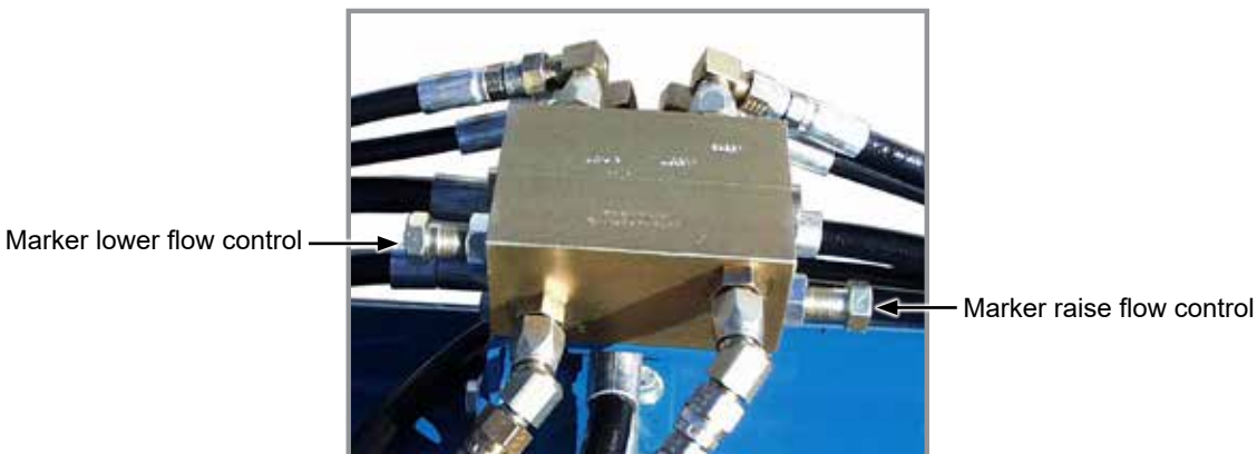
Row marker flow control valves
