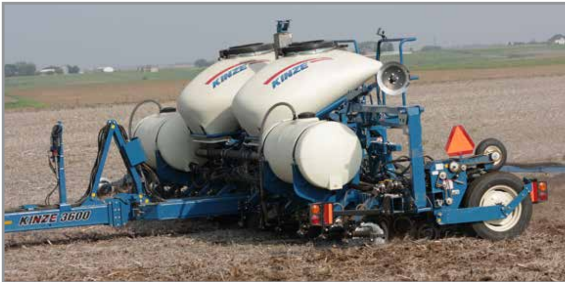
Liquid fertilizer installed on 3600 bulk fill
