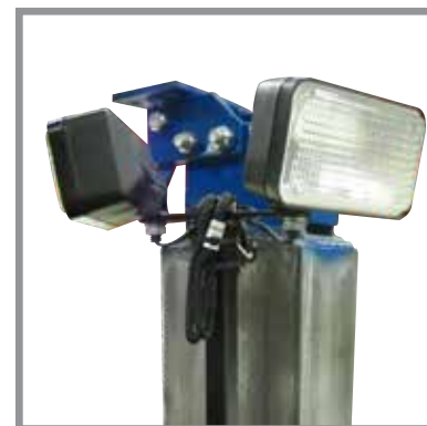
Auxiliary work lights
