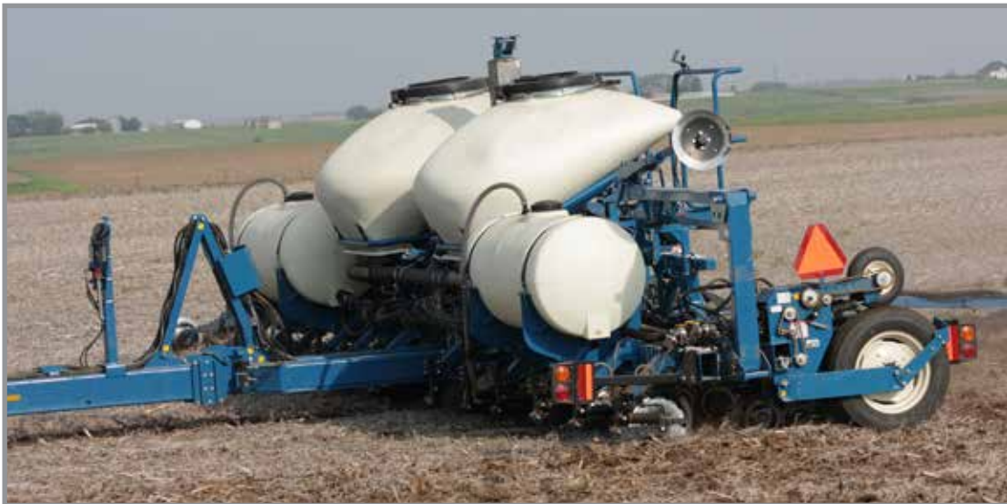
Liquid fertilizer installed on 3605 bulk fill
