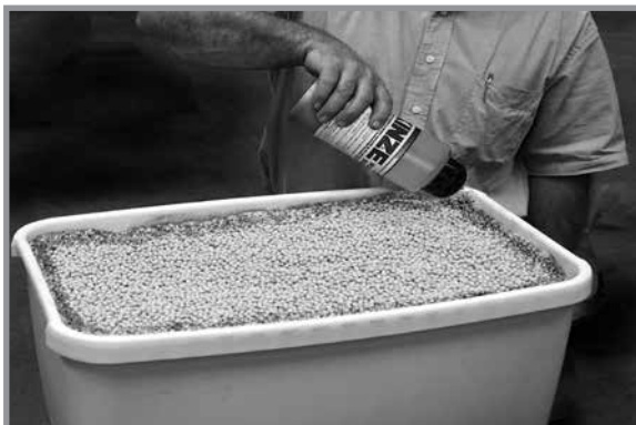
Adding graphite to conventional hopper
