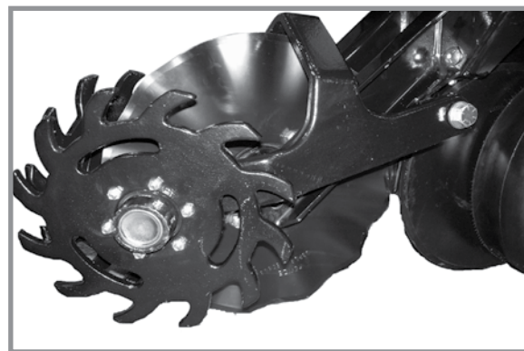
Coulters mounted residue wheels
