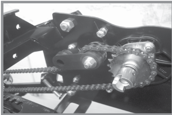
Mechanical push row unit meter drive
