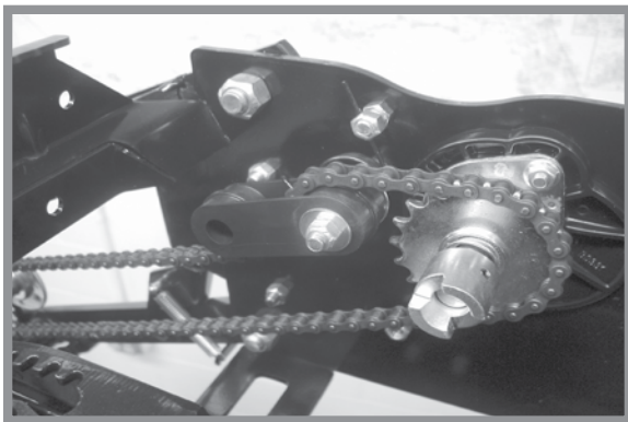
Mechanical push row unit meter drive
