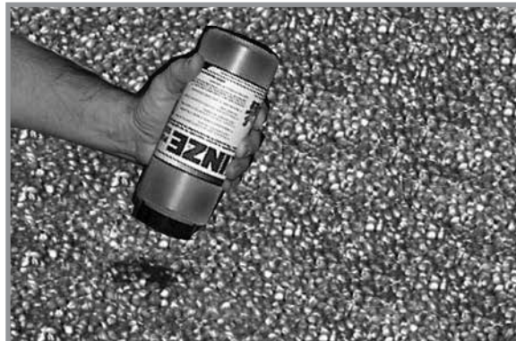
Adding graphite bulk fill hopper
