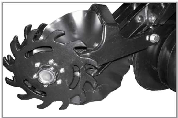
Coulter mounted residue wheels
