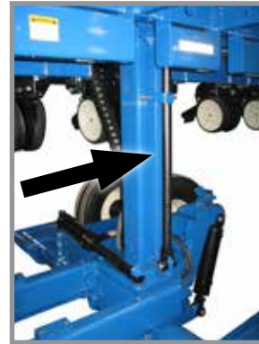
Safety lockup in transport/maintenance position
