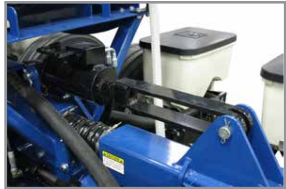
Wing lock engaged
