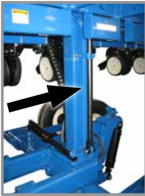
Safety lockup in transport position
