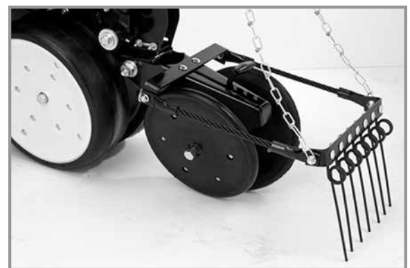
Spring tooth incorporator
