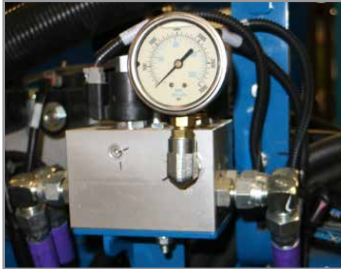
True Depth Pressure Gauge
