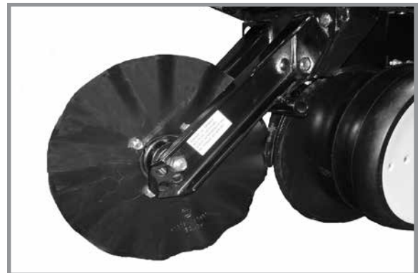
Row unit mounted no till coulters
