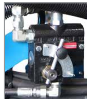
Flow Control Valve (True Depth)
