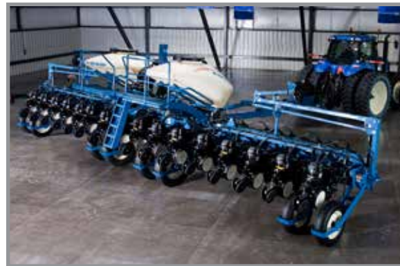
Planter in field lift position
