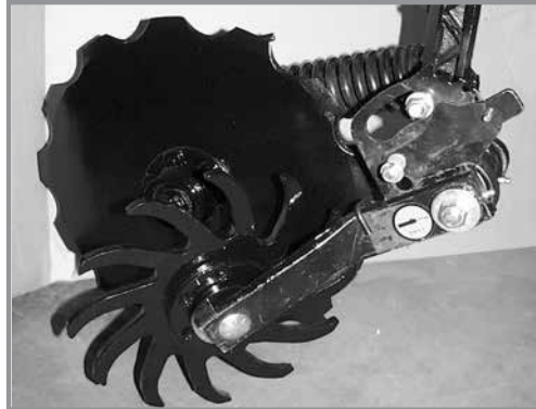
Notched single disc opener residue wheel attachment
