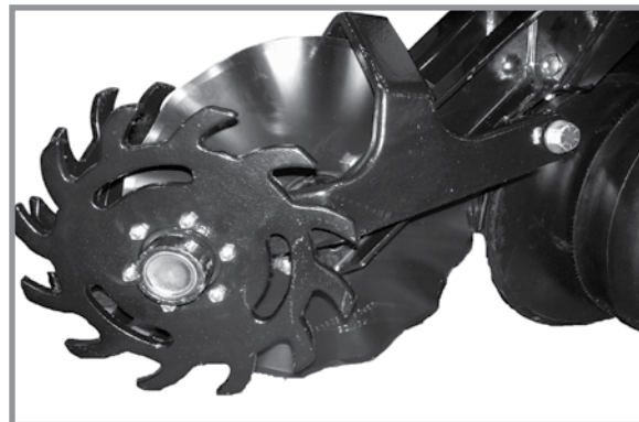
Coulters mounted residue wheels
