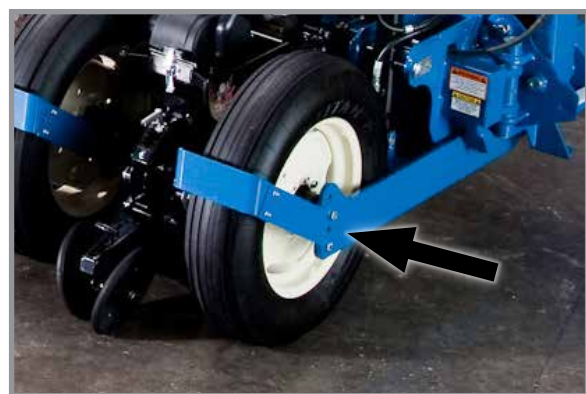
Field/wing wheel adjustment
