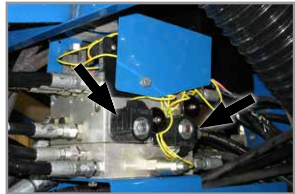
Row marker solenoid valves
