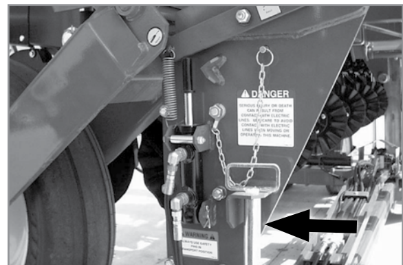
Tongue safety pin stored for field operation
