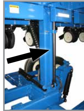
Safety lockup in transport/maintenance position
