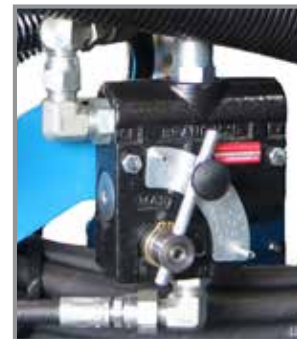
Flow Control Valve (True Depth)
