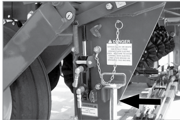
Tongue safety pin stored for field operation
