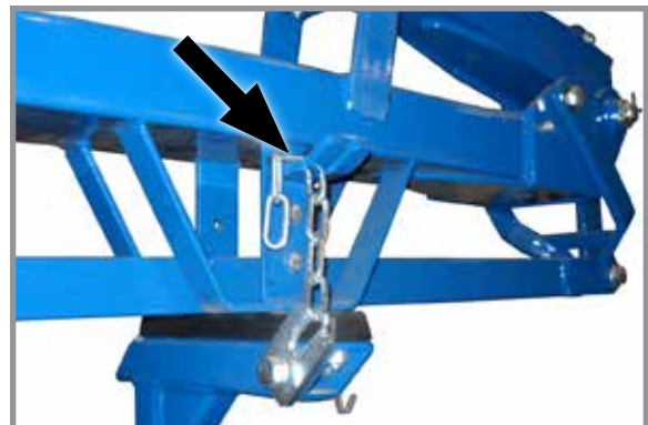
Row marker safety lockup installed
