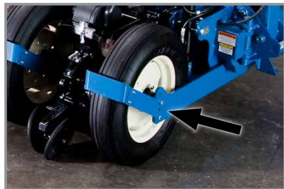
Field/wing wheel adjustment
