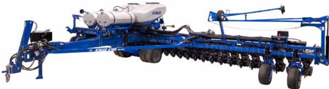
Model 4700 24 Row Bulk Fill Planter with Liquid Fertilizer
