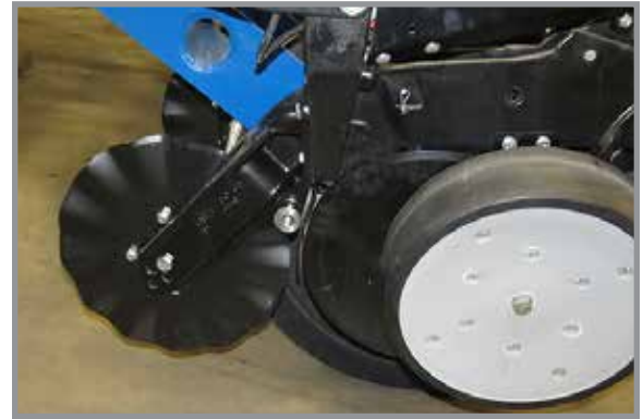
Row Unit Mounted No Till Coulters
