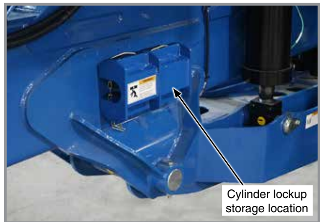
Cylinder lockup storage location
