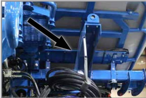
Cleanout Chute Storage Location
