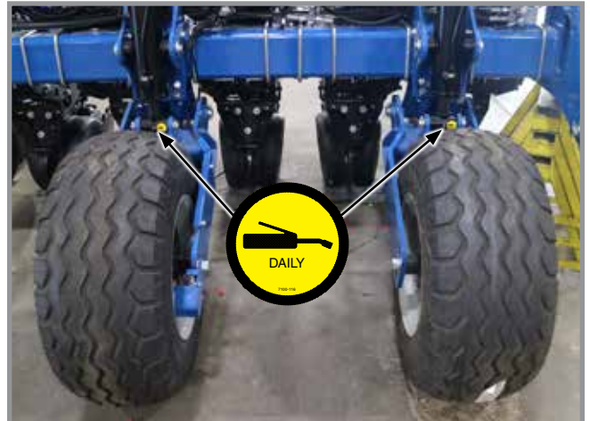
4. Lift Cylinders, 4 per machine 1 fitting per cylinder
