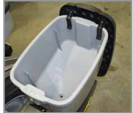
Granular Chemical Hopper
