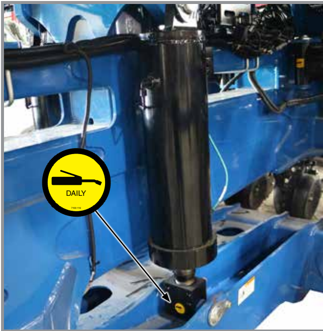
1. Lift Cylinder, 2 per machine 1 fitting per cylinder
