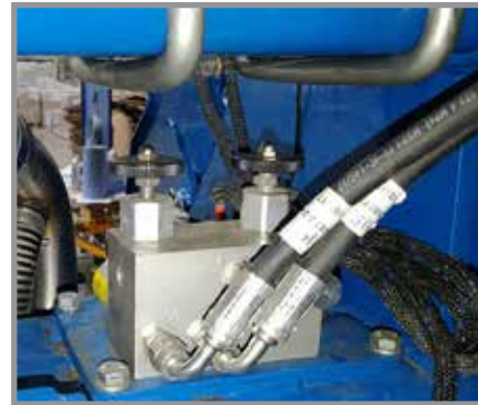
Row Marker Solenoid Valves
