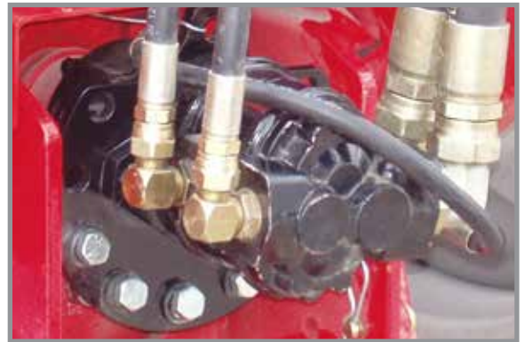
PTO Pump Installed
