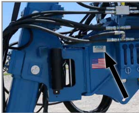
Serial Number Plate Location
