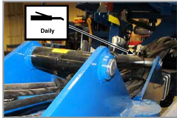
6. Wing Down Pressure Cylinder, 2 per machine 2 fittings per cylinder (one each end)
