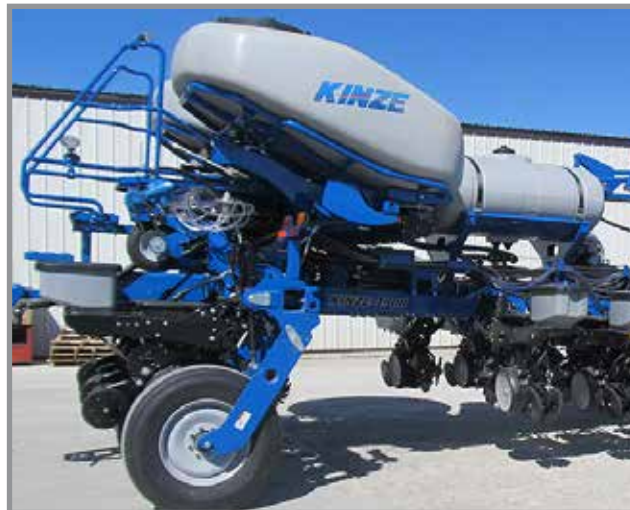
Liquid fertilizer installed on 4900 bulk fill
