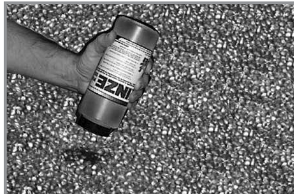
Adding graphite bulk fill hopper
