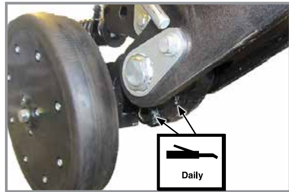
Grease to purge - 2 fittings
