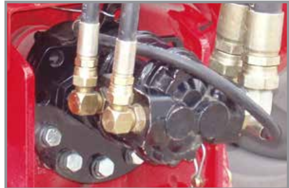
PTO Pump Installed
