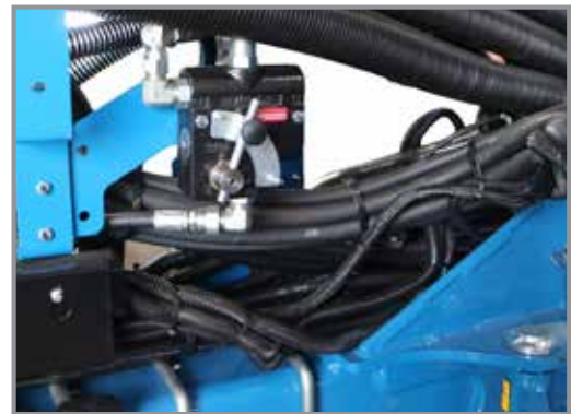
Flow Control Valve (True Depth)
