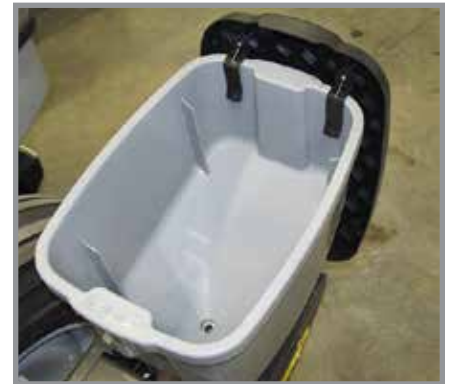
Granular Chemical Hopper
