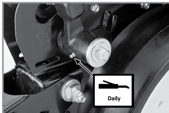
15. Gauge wheel arms - 1 per arm (Seals in gauge wheel arm are installed with lip facing out to allow grease to purge dirt away from seal. Pump grease into arm until fresh grease appears between washers and arm.)
