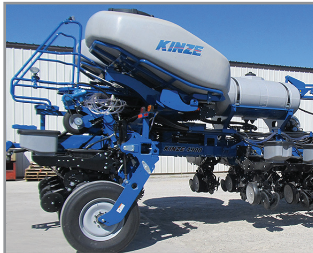
Liquid fertilizer installed on 4900 bulk fill
