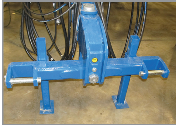
Jacks in Maintenance Position
