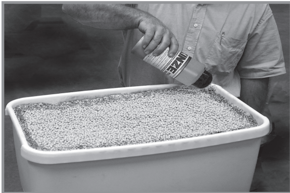
Adding graphite to conventional hopper
