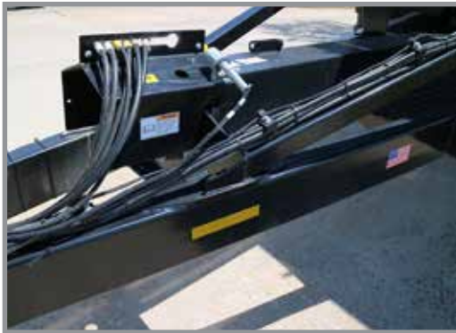
Hydraulic Hose Storage
