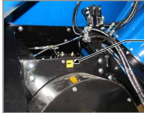
(2013-2017 Production) Rotate Bearing - 2 Zerks
