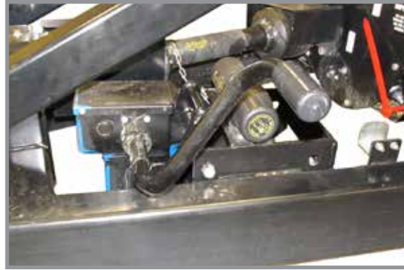
Jack handle installed
