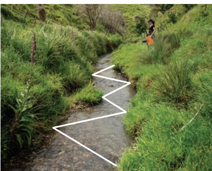
Very small (<2 m wide), wadeable stream: estimate periphyton cover at points along a zig-zag path that extends to the water's edge on each side.
