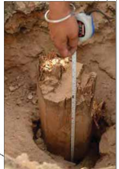
The wooden core at its point of snapping
