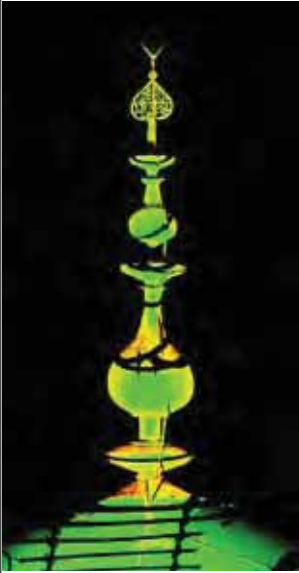
3D Laser Scanning, Architectural documentation of the finial listing out all the vessels and and Assessing the extent of damage on the finial due to the collapse
