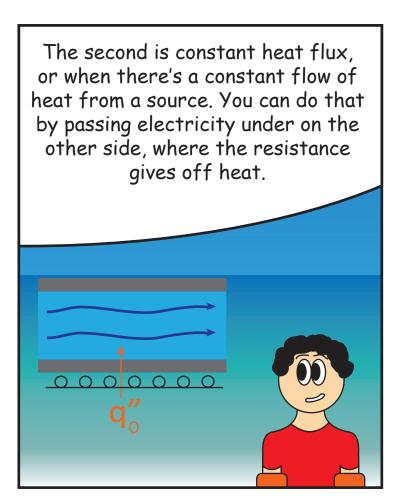
While the main concepts of convection are the same, most of the scenarios we talked about are isothermal. For constant heat flux, the equations are a bit differenct, but not harder.
