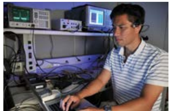
The Dynamic Spectrum Access Laboratory utilizes a Universal Software Radio Peripheral environment allowing scientists to conduct communications-based spectrum utilization and efficiency simulations prior to field testing.
