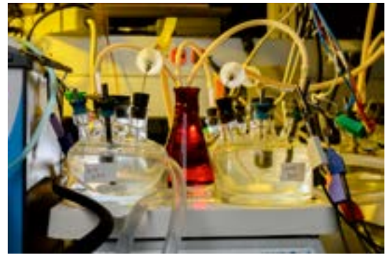
Microbial electrochemical reactors used to study electrode-microbe electrical interactions which are the basis of microbial electrochemistry and microbial electronics.
