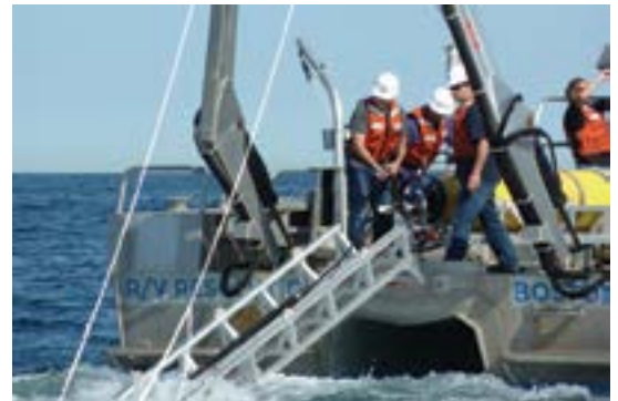
NRL's Reliant unmanned undersea vehicle with towed acoustic array is deployed during a long range active acoustics experiment.
