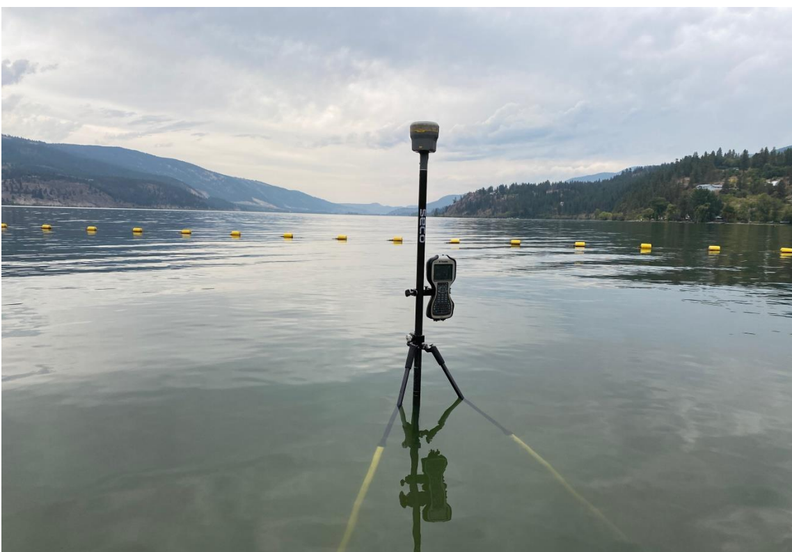
NV5 field survey photos showing water clarity conditions and ground survey equipment set up over submerged shallow water targets at two location within the Okanagan Lakes Area of Interest.
