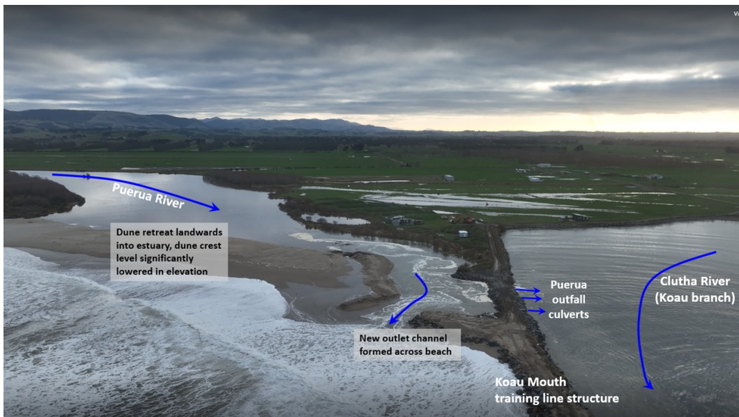
Figure 22: The coastline impact of the Puerua Estuary and Lower Clutha Flood Protection and Drainage Scheme infrastructure (5 July 2023).
