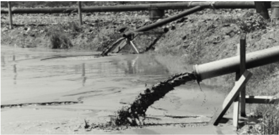
Tailings being dumped into the tailings dam at Vatukoula Gold Mine. Photo: Anne Lockley/Oxfam CAA
