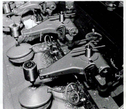
Automatic lens polishers. Hundreds of these units, large and small, are employed at Fuji's Omiya Factory.
