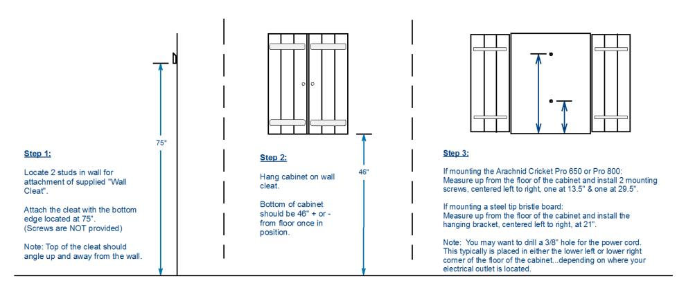
Tools needed: Level, cordless drill, 3/16" & 3/8" drill bits, screw tip.
