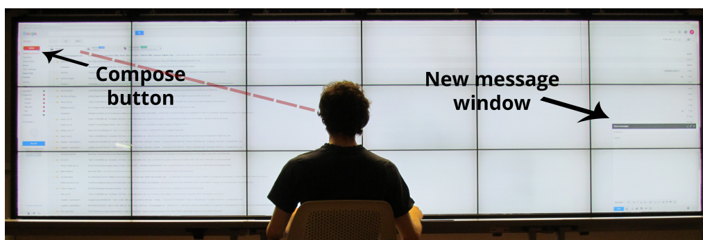
Figure 2.4: Gmail interface does not scale up well for a LVD. When the user presses the compose top left button, he cannot notice the new window on the bottom right because it is out of his field of view, as the red dashed line suggests.
