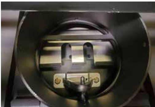
E- Upper Shield - orientation for reinstall
