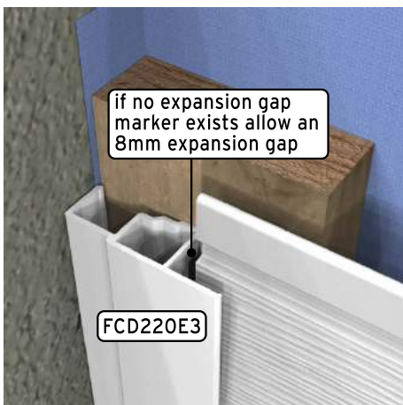
Typical Edge Detail - Multifunction Trim
