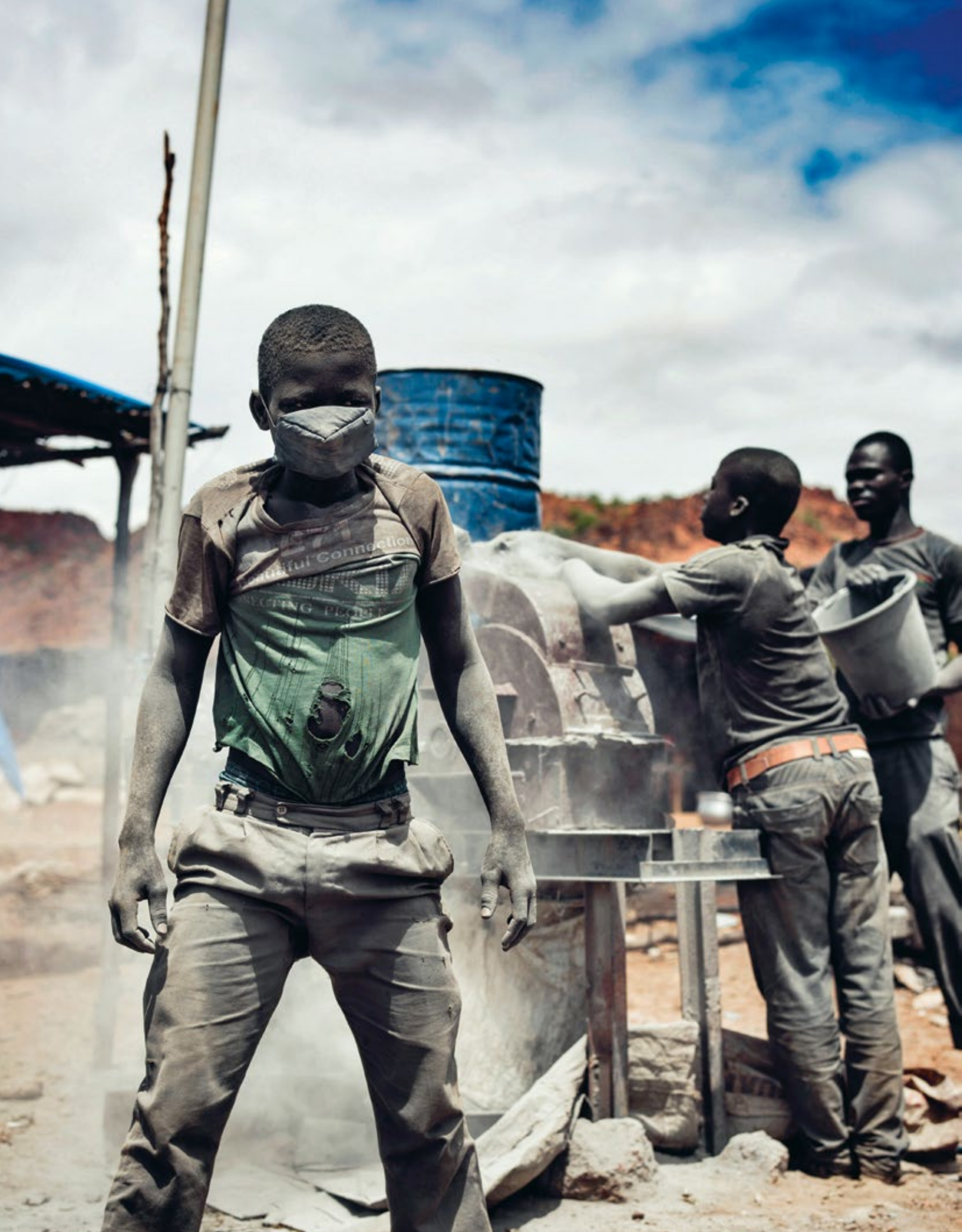
Adolescents operate machines that crush the smaller chunks of ore into dust for chemical treatment. Excessive dust exposure causes respiratory and pulmonary diseases. Workers migrate rapidly and independently depending on demand and the profitability of the mine site. // Alga mine site, 11th August 2015.
