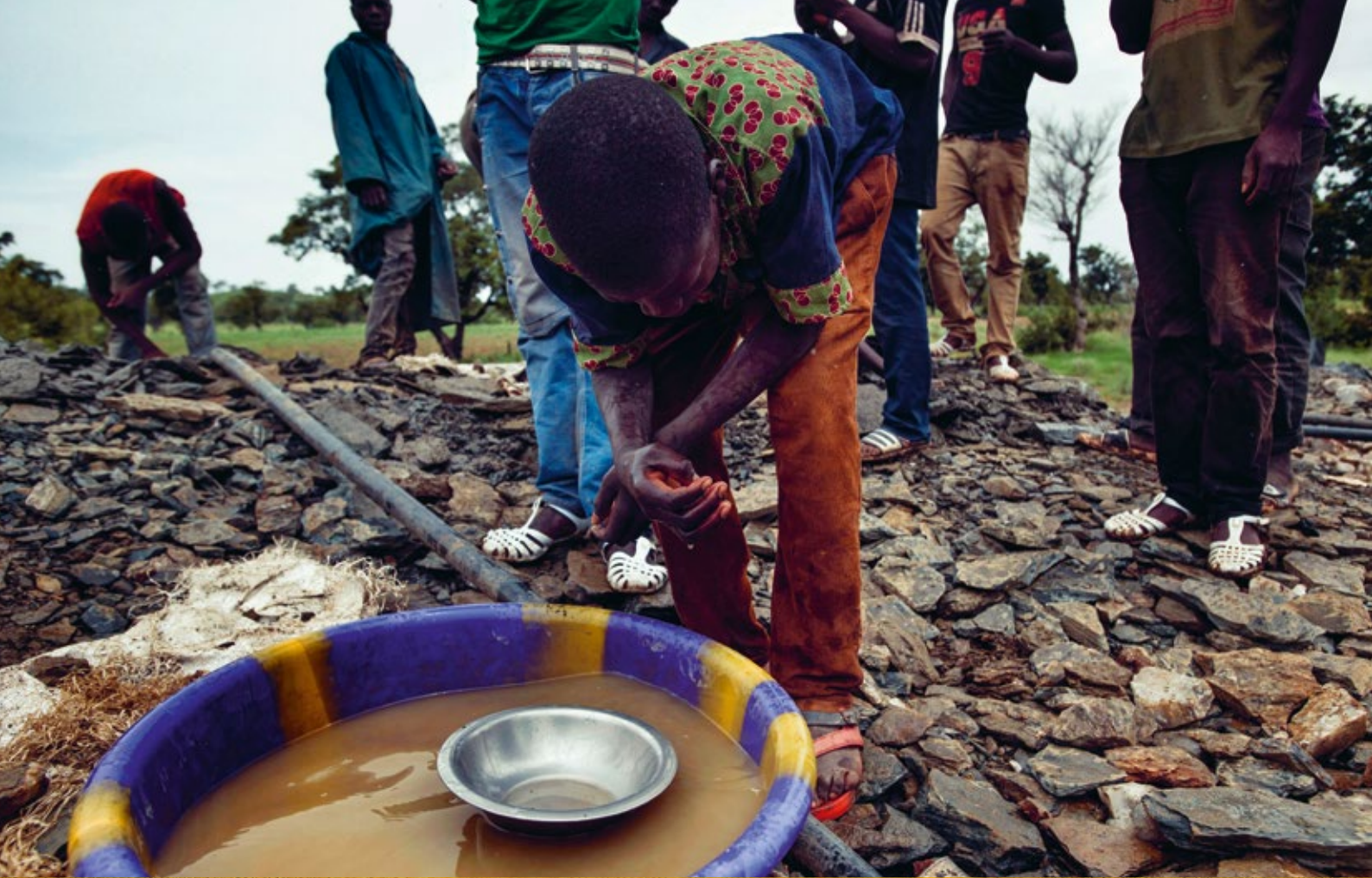
To separate the gold-bearing material from the silt, debris is washed and panned in sluice boxes. This is a task commonly undertaken by children. // Tikando mine site, 13th August 2015.
