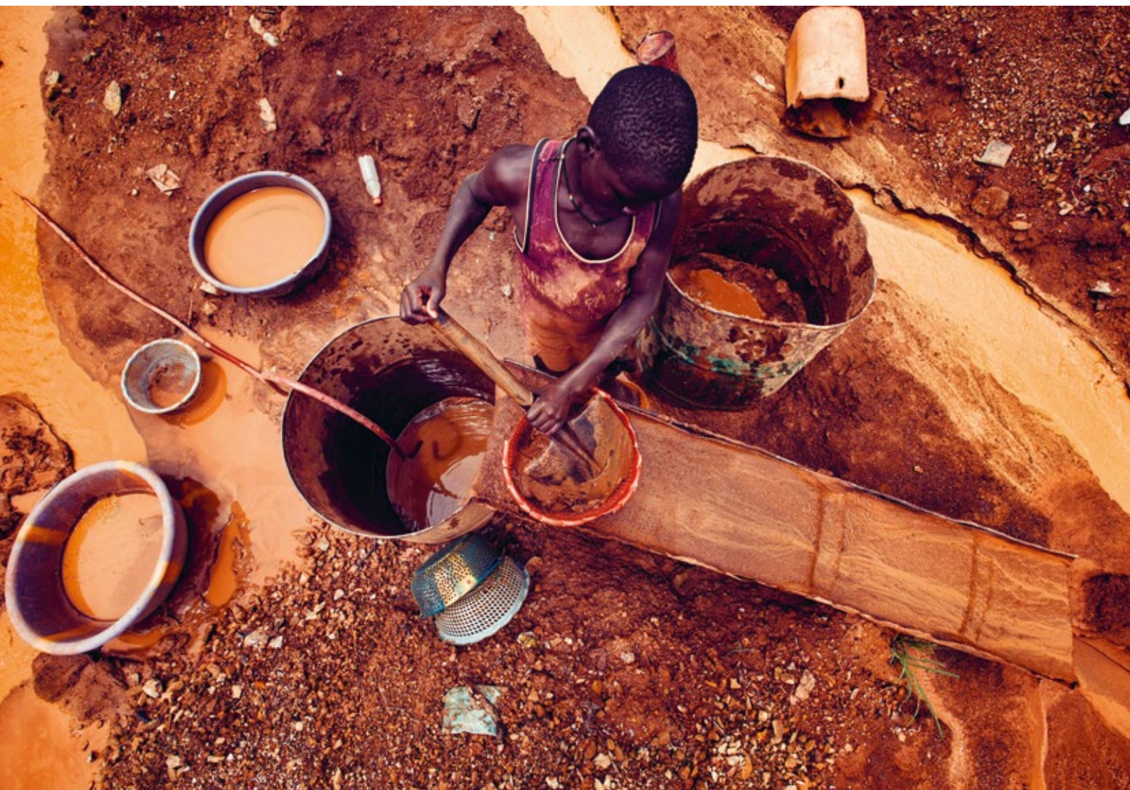
To separate the gold-bearing material from the silt, debris is washed and panned in sluice boxes. This is a task commonly undertaken by children. // Tikando mine site, 13th August 2015.
