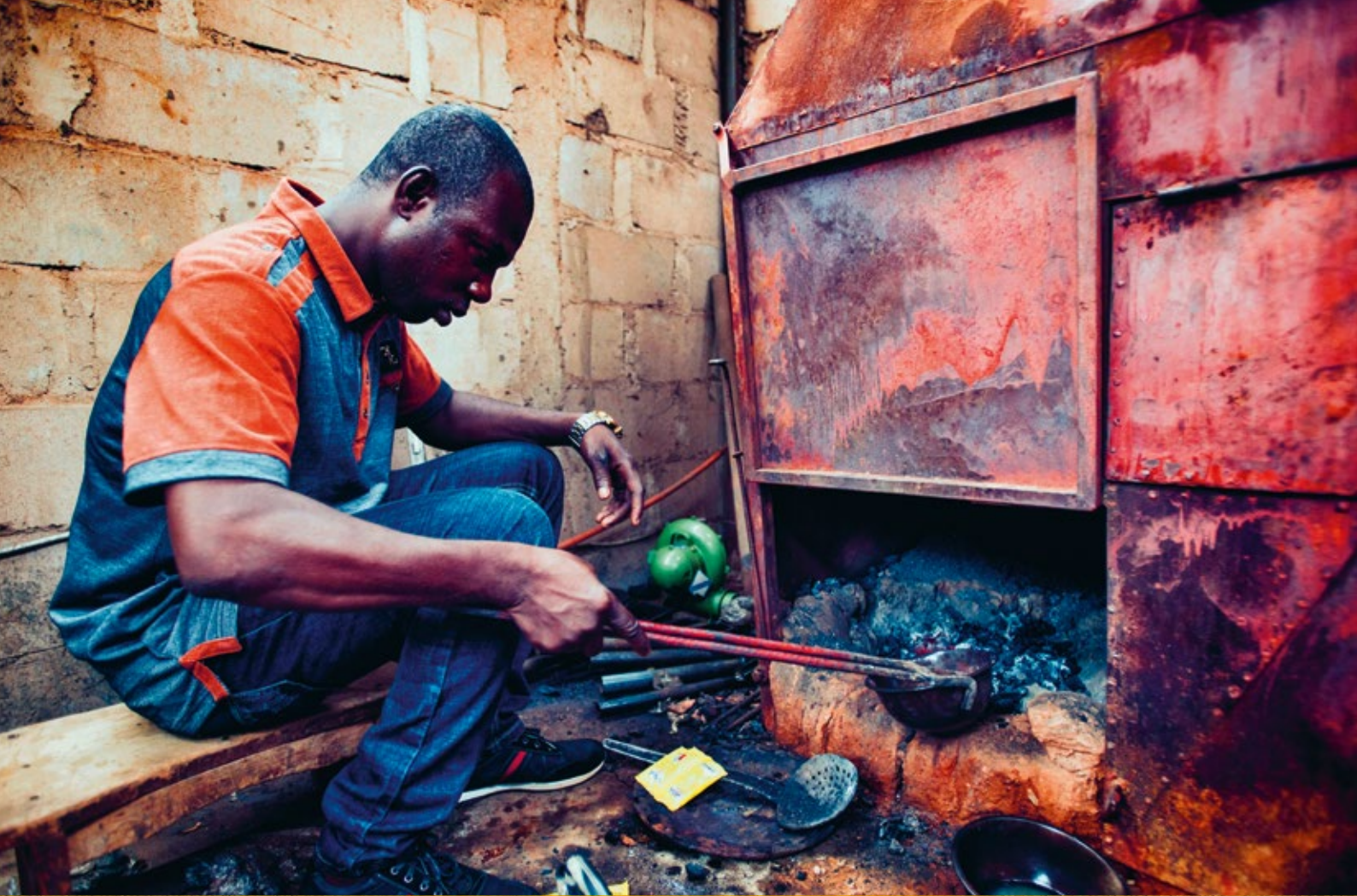
A small smelter is used on-site to pre-refine gold bars. // Kongoussi, 16th August 2015.
