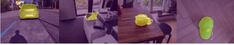
Figure 3: In some cases, geometry might not get recovered properly, as shown with the hole in the laptop. The hole in the handle of the teapot is not correctly inferred as free space. In the other two cases, some density is assigned outside of the object.
