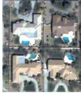
a) Quickbird true color b) Aerial Orthophoto visible size of the subset: 2 x 2 km, spatial resolution 0.61 m
