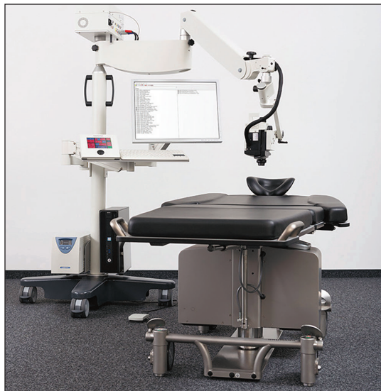
The Heidelberg Engineering Flex Module allows OCT imaging for patients in a supine position.
