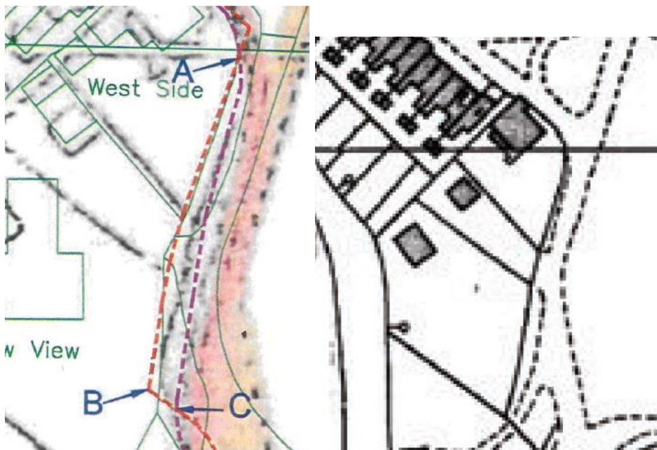
Figure 8: expert’s superimposition of conveyance plan line onto trace of 1971 OS plan; and 1971 OS plan extract
