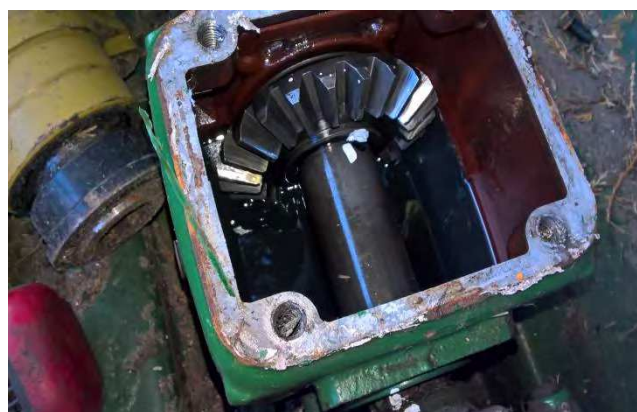
Figure 2 – Worn gearbox (Note mis-alignment of white marks)
