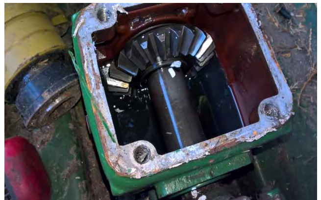
Figure 2 – Worn gearbox (Note mis-alignment of white marks)
