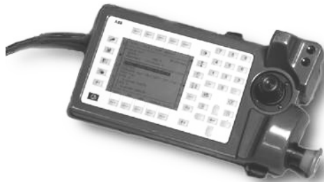
Figure 2.3 The teach pendant used for programming or manually moving the robot.
