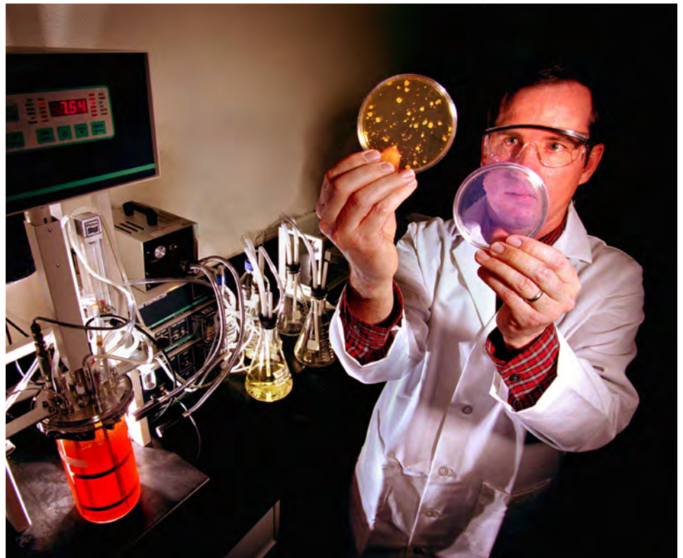
ANTICIPATING THREATS — In this 1999 photo, Sandia researcher Mark Tucker examines two petri dishes: one with a simulant of anthrax growing in it, left, the other treated with the decontaminating formulation developed at Sandia.
