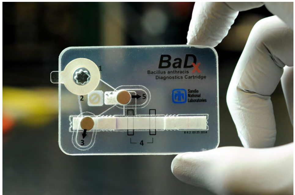
POCKET TEST — The BaDx pocket-sized detector has everything needed to test a sample for anthrax. It is a safer, easier, faster and cheaper testing solution for resource-constrained parts of the world.
