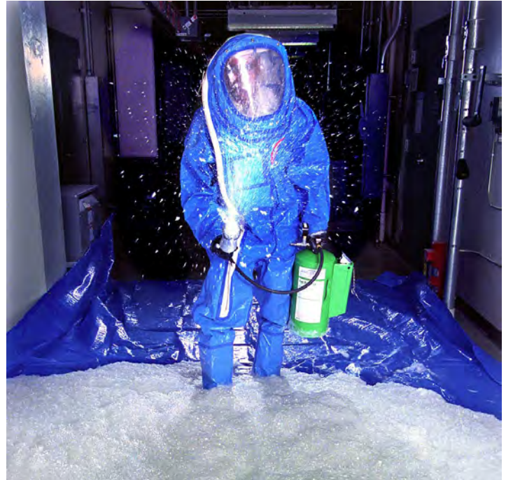
TIME TO SHINE — Former Sandia researcher Maher Tadros demonstrates application of decontamination foam, which was deployed on Capitol Hill, in mailrooms and in newsrooms during the anthrax scare following 9/11. Tadros and researcher Mark Tucker co-developed the foam in the late 1990s.
