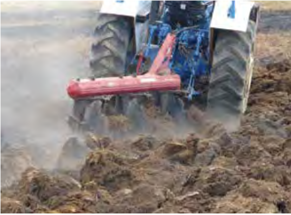
Figure 16.5. Left: A heavy disk (disk plow) can be used for primary and secondary tillage. Photo by Mark Brooks. Right: A finishing disk.
