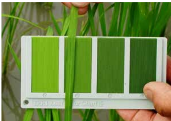
Figure 21.6. International Rice Research Institute (IRRI) leaf color chart for nitrogen evaluation with rice. Photo by IPNI.
