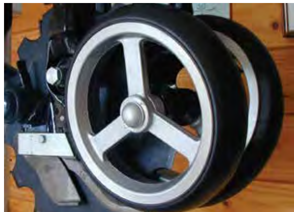
Figure 16.8. Left: A no-till seed drill requires no-till or seedbed preparation for narrow-seeded crops or cover crops. Right: The cross-slot opener used in no-till planters. The disk slices soil, the inverted T blade allows seed and fertilizer placement on opposite ends of the disk, and the packer wheels (right side) close and firm the seedbed.
