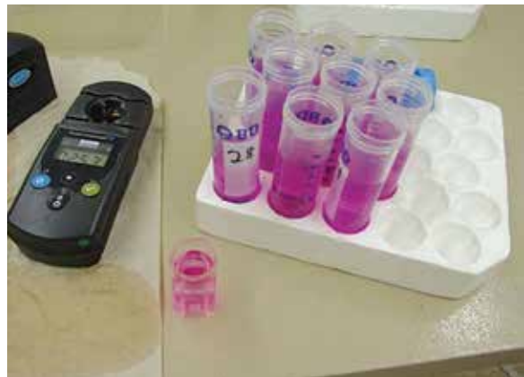
Figure 23.7. Assessment of active carbon using permanganate oxidation and a portable spectrophotometer. Photo by David Wolfe.
