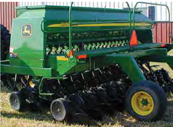
Figure 16.8. Left: A no-till seed drill requires no-till or seedbed preparation for narrow-seeded crops or cover crops. Right: The cross-slot opener used in no-till planters. The disk slices soil, the inverted T blade allows seed and fertilizer placement on opposite ends of the disk, and the packer wheels (right side) close and firm the seedbed.
