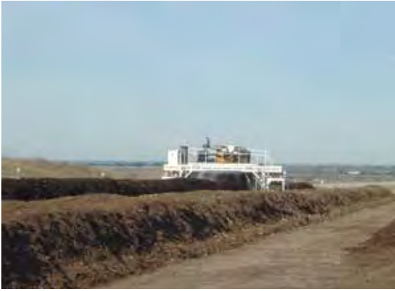
Figure 13.3. Turning a compost windrow at a commercial facility. Photo by Alison Jack.
