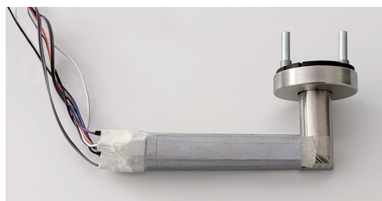
Figure 1: The final prototype from our door handle with the lengthwise attached sensor stripes. The positions of the sensor stripes are Top, Bottom, Back and Front.
