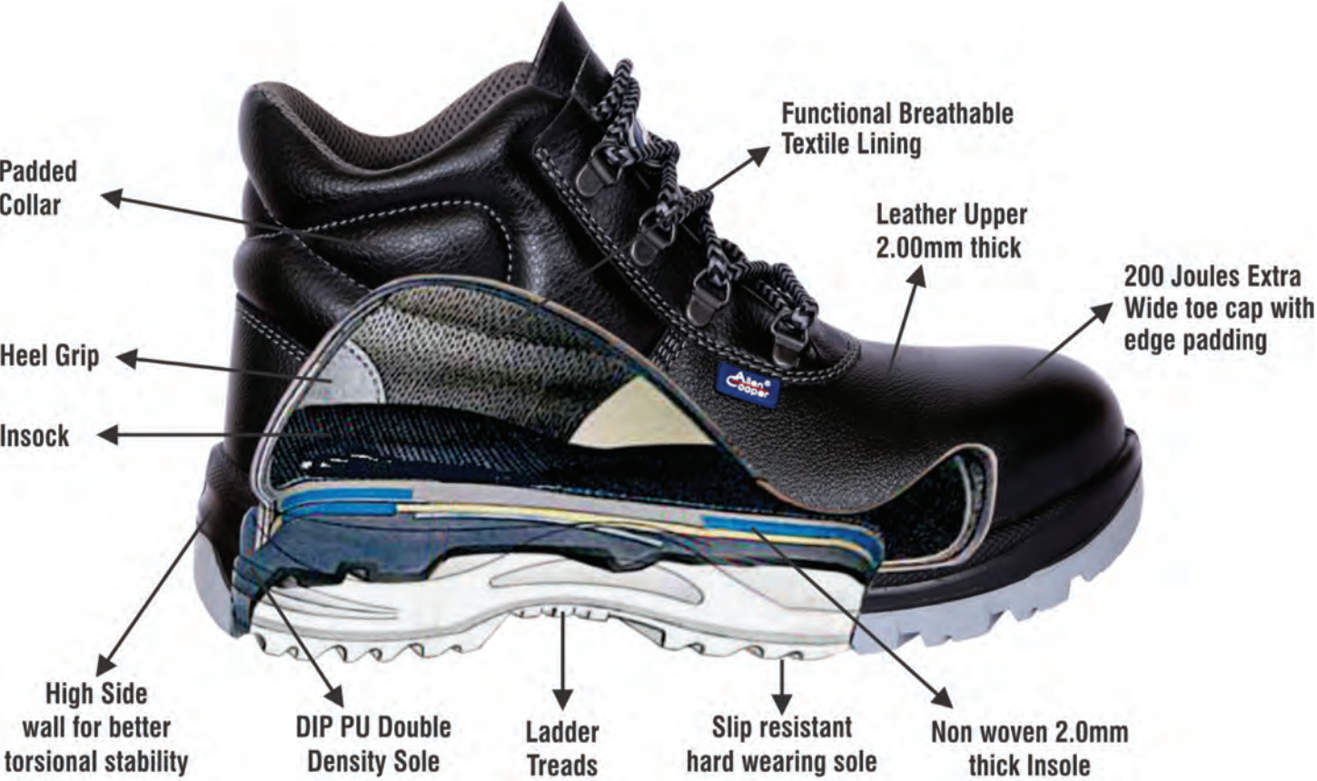
Diagram of Typical Safety Shoe (with Anti-penetration insole)
