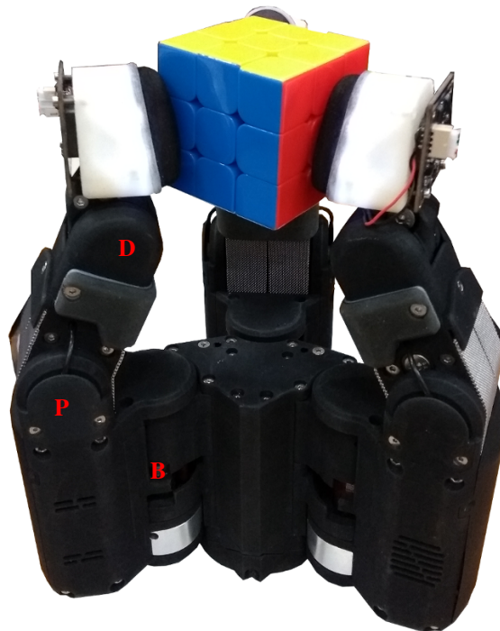
Fig. 1: Image of the developed tactile sensors integrated with the Shadow Modular Grasper. Base, proximal and distal joints are labelled B , P and D respectively.
