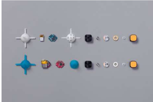
(a) The components of the Giiker cube.
