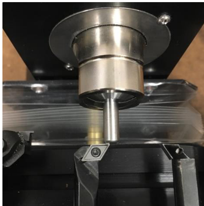
FIGURE 15—Notice the carbide tip on the left just touching the front of the dowel
