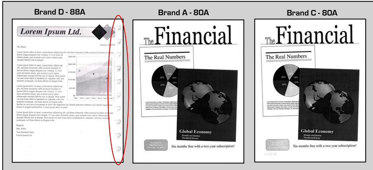
Images magnified to show Print Quality defect. Images may not be accurately reproduced when printed from this report.
