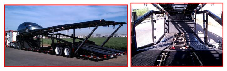
This high mount style stacker helps any road tractor navigate small yards and city streets yet maximizing your load. You can add flip-out extensions or a tilt deck on the bottom for additional load space as well as a shotgun to load a head rack on your power unit.
