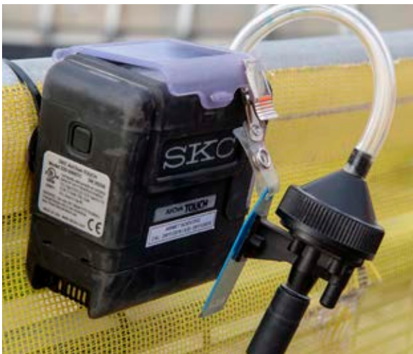
Static monitoring in place on Central Station measuring respirable dust and respirable crystalline silica
