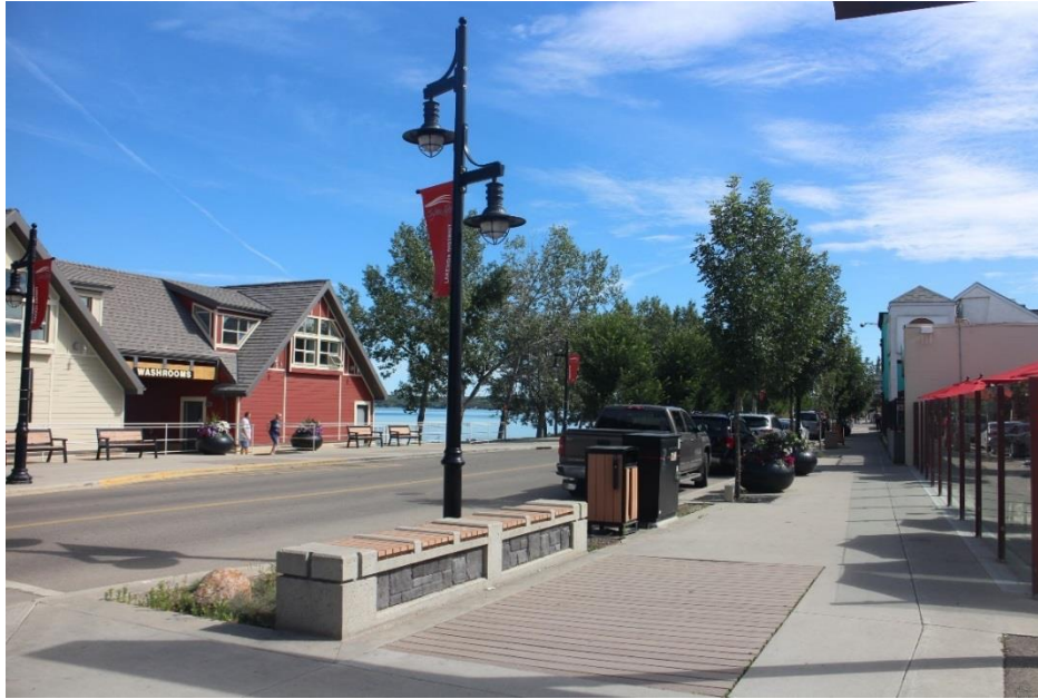
Figure 4: The wide sidewalk is buffered from vehicular traffic by boulevard trees, planters, stylized light stands, and benches. The roadway is narrowed by the bump outs at pedestrian crossings, effectively slowing vehicular traffic.
