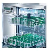
Cleaning processes can be referred to as batch or in-line processes. Batch systems refer to a batch of PCBs taken through the entire process, whether it is ultrasonic or dishwasher application, for example. Cleaning processes can also be set up as in-line systems where PCBs are constantly transferred through each stage and a continuous production line is formed.
