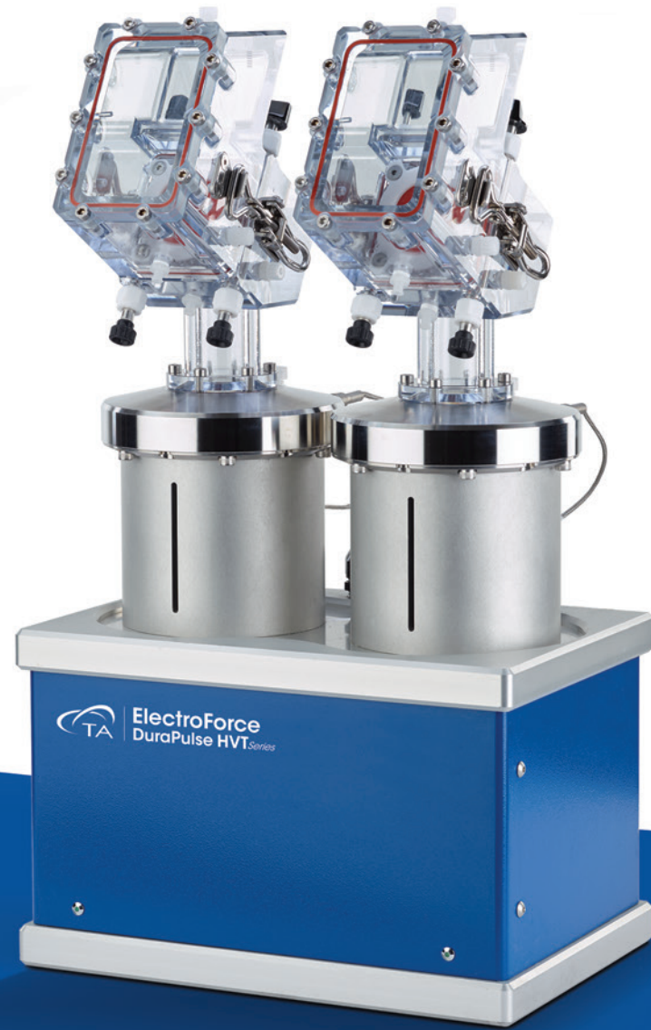
Accelerated wear testing of complete heart valve device
