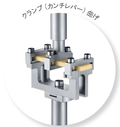
ABS bar - Cantilever 3 mm x 12.75 mm x 25 mm
