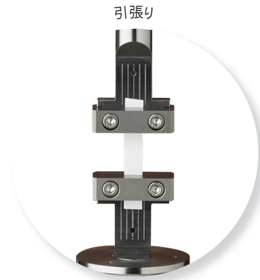
PET Film - Tension 50 μm thick
