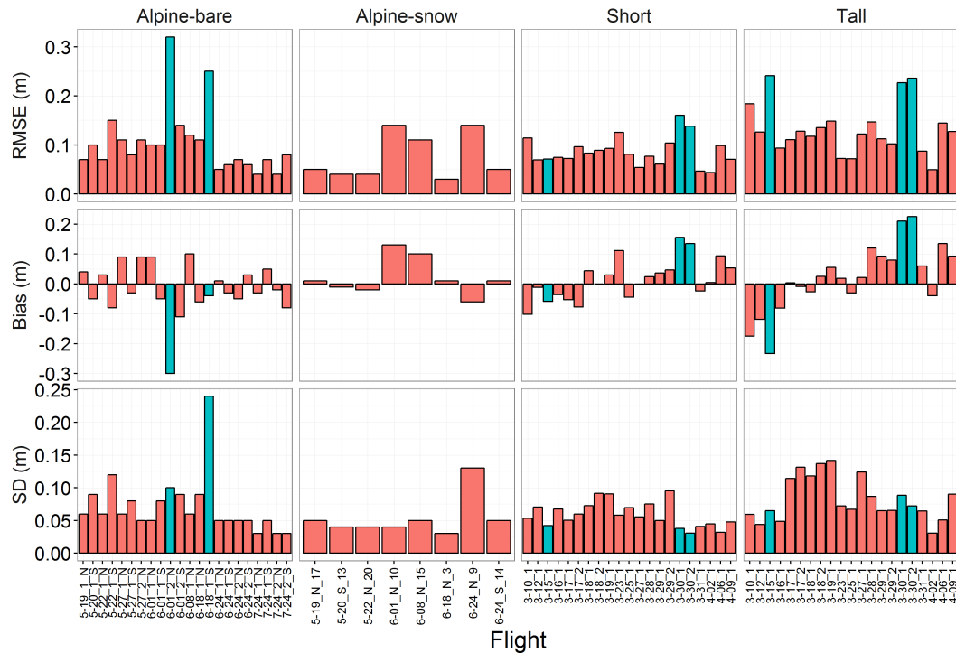
Figure 4. Root mean square error (RMSE, top row panels), bias (middle row panels) and standard deviation (SD, bottom row panels) of DSMs with respect to surface over alpine-bare, alpine-snow, and short and tall stubble at prairie site, respectively. Blue bars highlight problematic flights and are excluded from summarization in Table 2. The x axis labels represent month–day–flight number of the day (to separate flights that occurred on the same day). Alpine-bare accuracies are separated into northern or southern areas, reflected with an N or S suffix. The last number in the alpine-snow x axis label is the number of observations used to assess accuracy as the number of surface observations varied between 3 and 20.
