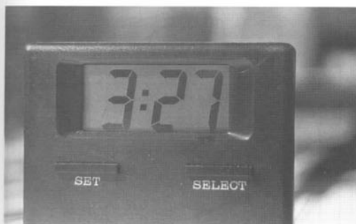
Fig. 2-1. Analog measures continuously; digital measures in steps, and each step is exact.
