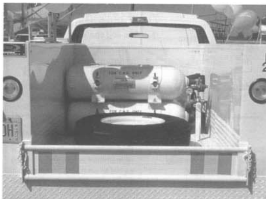
Fig. 3-4. NG first usage is more likely on trucks because NG tanks are bulky.
