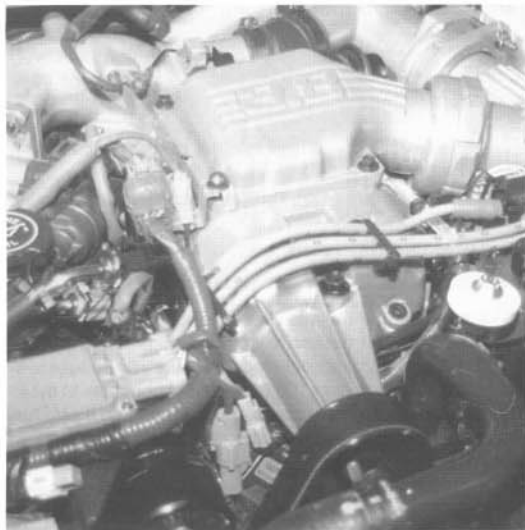
Fig. 3-8. Engine-driven supercharger in 3.8L Ford delivers better low-speed torque than exhaust-driven turbocharger.
