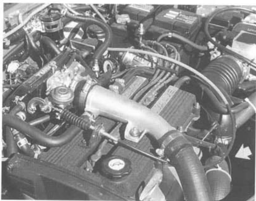
Fig. 3-7. Engine exhaust drives the turbocharger (arrow). Ford uses turbochargers on some 1988 and later and some MECS engines.
