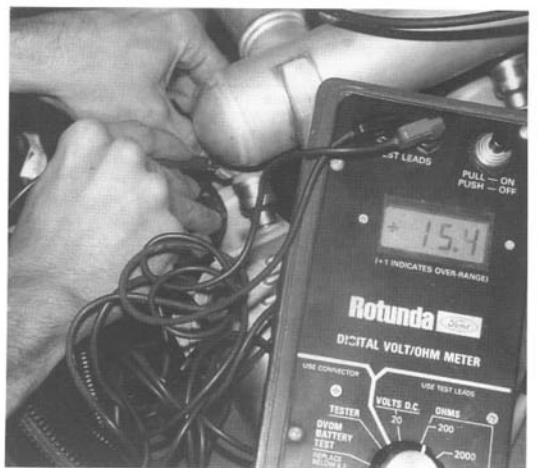
Fig. 2-13. Checking injector resistance.
