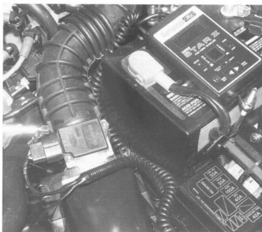
Fig. 4-14. In Continuous Monitor Test (EEC-IV only) you attempt to recreate fault while checking for codes. For example, tap MAF sensor while watching STAR tester.
