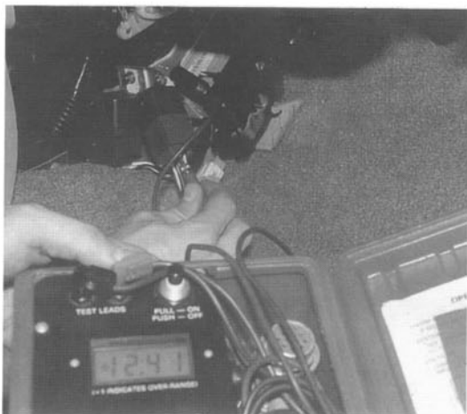
Fig. 2-6. Check voltage at fuel-pump relay. On the '91 1.9L Escort, it is under the center console.
