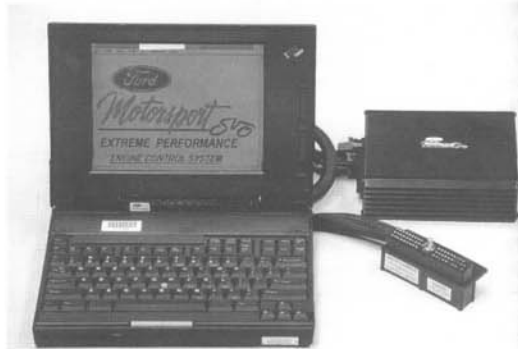
Fig. 6-16. Ford EPEC system installs between EEC-IV module and wiring harness and interfaces with a laptop computer to give total control over the calibration of air-fuel ratio, spark, and other parameters.
