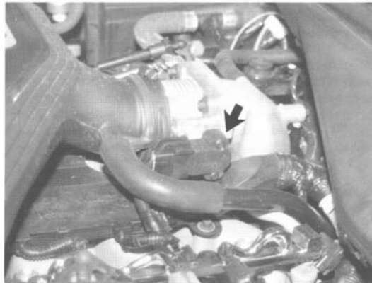
Fig. 7-1. Throttle Position (TP) sensor (arrow) sends a feed-forward signal to control module of just what you would expect—throttle position. Movement signals what driver expects engine to do.
