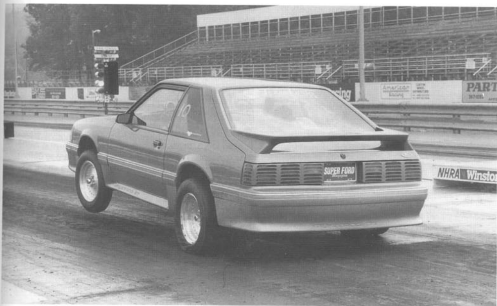
Fig. 6-17. This 1989 Mustang GT hatchback pulls an 11.94 quarter mile at 113.26 mph. Modifications include GT-40 intake with 65mm throttle body and the stock MAF sensor ported to 61mm.
