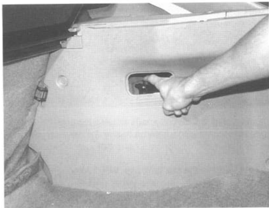
Fig. 2-8. Inertia switch in trunk.
