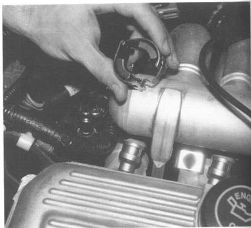
Fig. 2-10. You'll need special Ford tool to open fuel lines.
