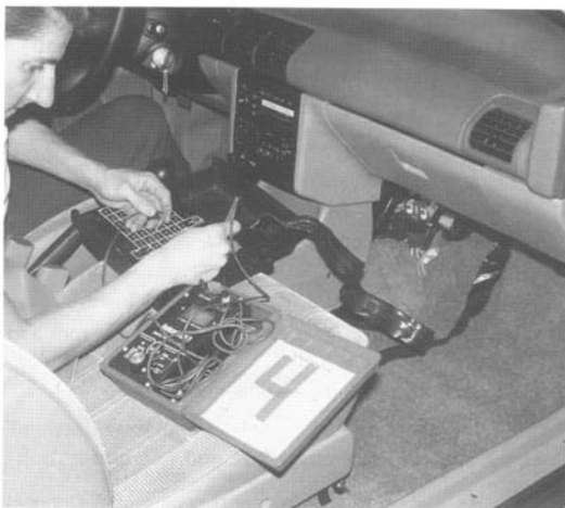
Fig. 4-5. Check DIS/EDIS inputs to EEC control module (PIP, IDM) at control module connector using BreakOut Box (BOB).
