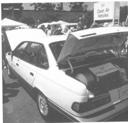
Fig. 3-7. Ford Taurus converted to dual fuel, capable of operating on NG (Natural Gas) without fuel injection, or gasoline.
