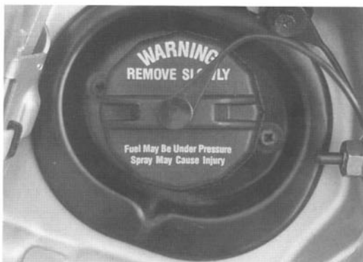
Fig. 2-7. Ford sets relief valve in the fuel tank cap at 1.6 psi (11 kPa). That small pressure can force fuel out of an open return line.
