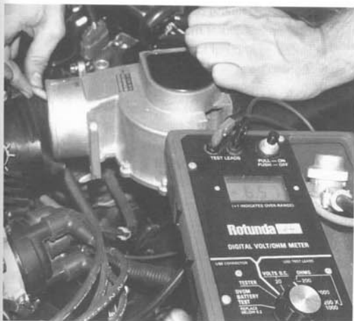
Fig. 3-4. Place a pencil through the VAF to deflect the vane. Measure the voltage output. Shown is 2.2L Turbo.
