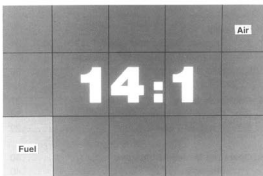
Fig. 2-2. It takes about 14 parts of air by mass to support complete combustion of 1 part of gasoline fuel. Once upon a time, an air-fuel ratio somewhere close to 14:1 was good enough.
