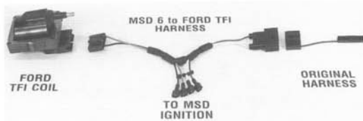
Fig. 6-19. Motorsport MSD kit provides simple installation of control unit to Ford TFI coil.
