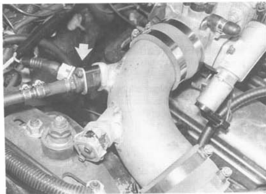
Fig. 7-3. Add-on fuel injector (arrow) can supply fuel for high demand situations, but precise control of air-fuel ratio is difficult.
