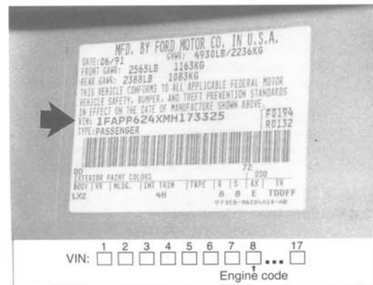
Fig. 2-11. Vehicle Identification Number (VIN) on door jamb. Look at eighth digit to determine engine code.
