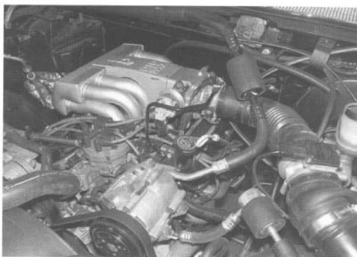
Fig. 6-4. GT-40 intake manifold (here with 65mm throttle body) can mean big horsepower gains. By themselves they are not street-legal, but Ford sells a full GT-40 kit (including valve train components, heads and ring and pinion set) that is 49-state legal.
