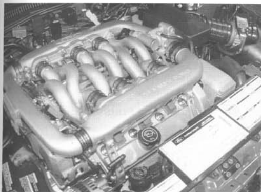
Fig. 2-4. SHO 3.0L engine in 5-speed transaxle (M/T) Taurus delivers 220 horsepower from 3.0L. Beginning '93, SHO 3.2L 220 bhp comes with automatic transaxle, E4OD.
