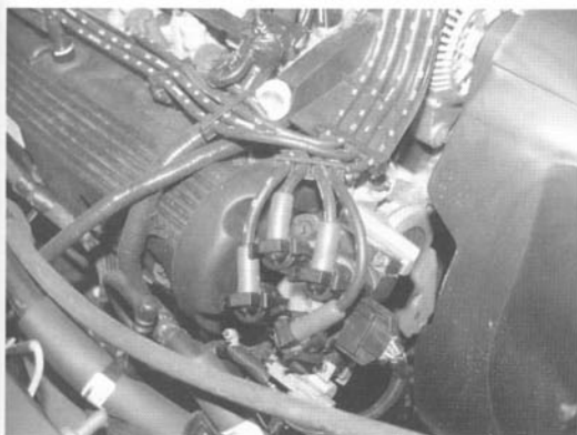
Fig. 3-14. Coil pack on each cylinder bank of 4.6L V-8 shows plug wires crossing to other bank, necessary to fire cylinders in proper pairs.
