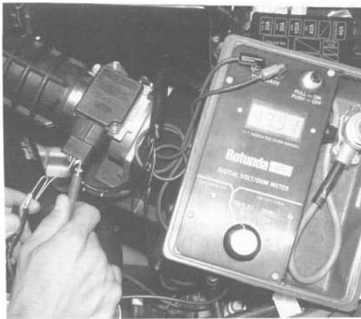
Fig. 1-1. Backprobing gives you access to circuit signals without breakout box. Checking VPWR to Mass Air Flow (MAF) sensor shown. Take care not to damage connector or terminals.
