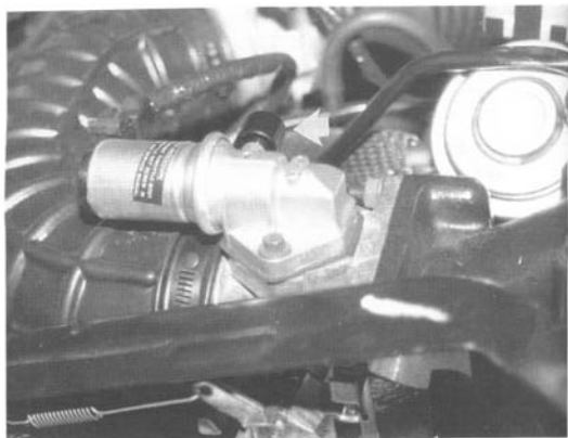
Fig. 4-4. If you see vent filter (arrow), you know this is a different Hitachi unit that cannot be cleaned.
