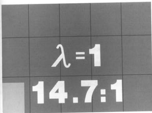
Fig. 5-2. For warm gasoline-fueled engines at part throttle, most complete combustion occurs at ideal (stoichiometric) air-fuel ratio of about 14.7:1—approximately 14 kg air for every 1 kg fuel.
