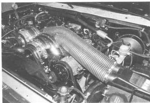
Fig. 6-11. Paxton twin-supercharger kit for large-displacement engines provides over twice the volume of air over single 5.0L unit. Kit pending CARB exemption.
