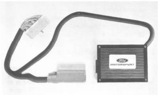
Fig. 6-15. SVO Extender is extra control module that installs between EEC-IV module and wiring harness to give additional air-fuel ratio control and redline adjustment.
