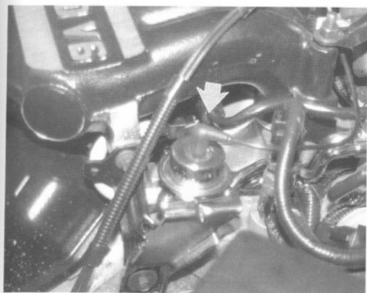
Fig. 3-1. Pressure regulator (arrow) at end of fuel rail controls fuel pressure by controlling fuel return flow to tank. Hose connection leads to intake manifold.
