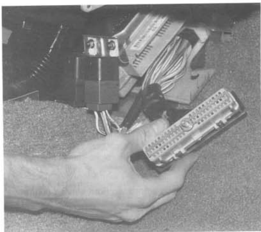
Fig. 2-1. Connectors, harnesses and grounds are common trouble spots in electronic engine-control systems. Make sure connections are clean and tight. In earlier systems, cleaning corrosion from connectors will often fix problems without replacing components.
