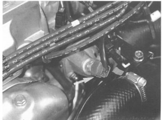
Fig. 5-1. Engine Coolant Temperature (ECT) sensor is located in coolant system in heater outlet fitting, near flywheel in 2.3L, and 3.8L Taurus/Sable and Continental; opposite flywheel in others.
