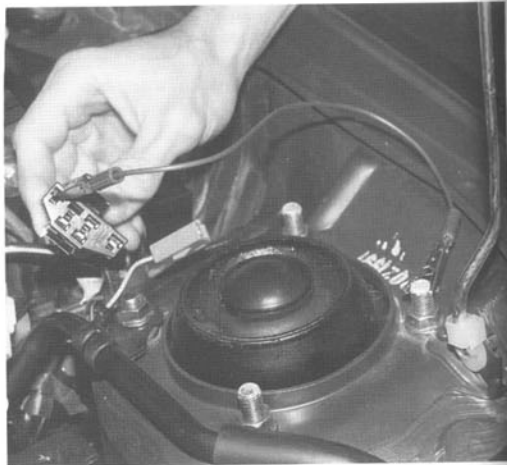
Fig. 2-2. Grounding Fuel Pump (FP) lead of Self-Test Connector to run fuel pump with engine off.
