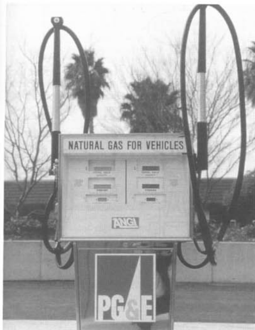
Fig. 3-3. Experimental NG fuel pumps provide fill-ups, but must supply fuel through special fittings under pressure as high as 3,000 psi (21,000 kPa).
