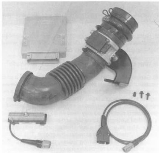
Fig. 4-1. Mass Air Flow (MAF) kit converts Manifold-Absolute Pressure (MAP) direct sensing of air-flow to direct system for performance mods. Includes new EEC-IV control unit.
