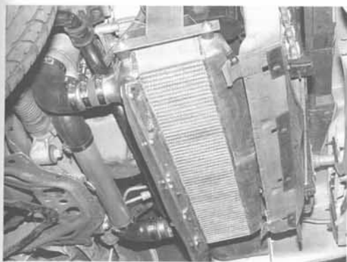
Fig. 6-8. Intercooler from Spearco is designed to work with 5.0L Supercharger kit from Vortech.
