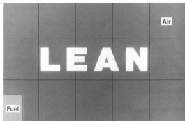
Fig. 2-4. A lean mixture burns almost all the fuel, so exhaust gas contains leftover oxygen, and very little unburned gasoline.
