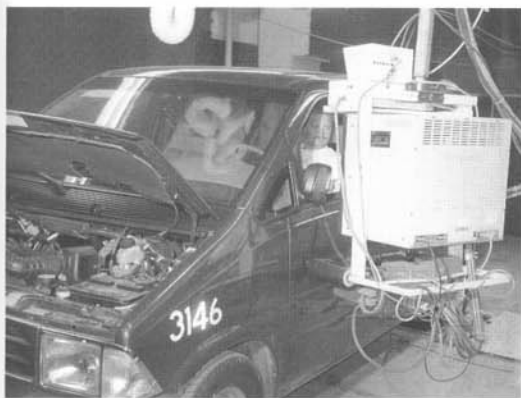
Fig. 2-3. Every car and light truck engine is certified to meet EPA emissions standards, and from those measurements, standards for fuel economy. Drivers follow exact driving pattern. Dynamometer rolls load engine according to inertia weight and resistance to movement, including friction, tire rolling resistance, and aerodynamic drag.
