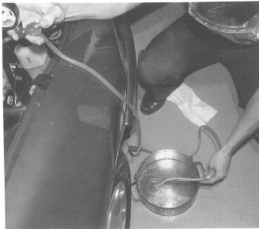
Fig. 2-4. Check return flow from regulator. Fuel-pressure gauge fitted to Schrader valve has drain valve.
