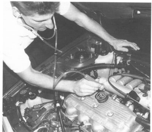
Fig. 2-12. You can check injector operation with a stethoscope or by placing screwdriver tip against injector body and listening for clicking sound.
