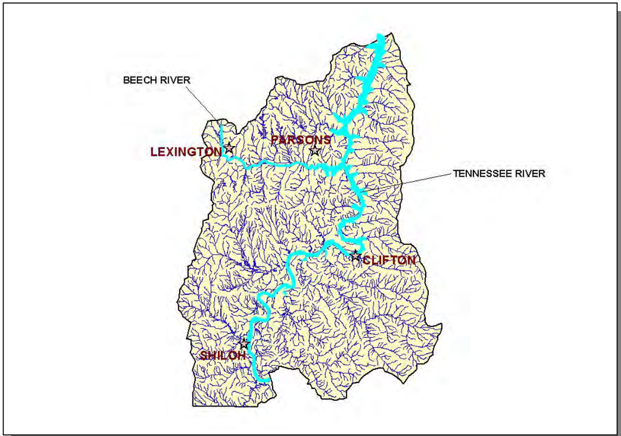
Figure 2-4. Hydrology in the Tennessee Portion of the Tennessee Western Valley (Beech River) Watershed. There are 3,435 stream miles and 20,763 lake acres in the Tennessee portion of the Tennessee Western Valley (Beech River) Watershed as catalogued in the assessment database. An additional 88 stream miles are located in the Mississippi portion of the watershed as catalogued in the River Reach File 3 database. The Tennessee River and Beech River, and the cities of Clifton, Lexington, Parsons, and Shiloh are shown for reference.
