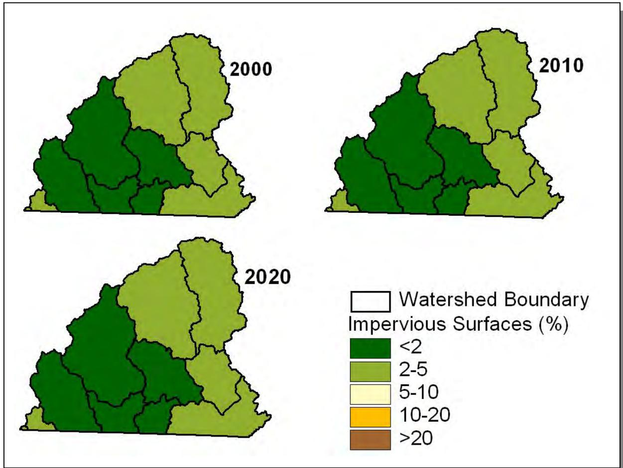
**Figure 2-9. Illustration of Total Impervious Area in the Tennessee Portion of the Guntersville Lake Watershed.** All HUC-12 subwatersheds are shown. Current estimates and projected total impervious cover calculated by HUC-12 are provided by EPA Region 4. More information can be found at: <http://www.epa.gov/ATHENS/research/impervious/>
