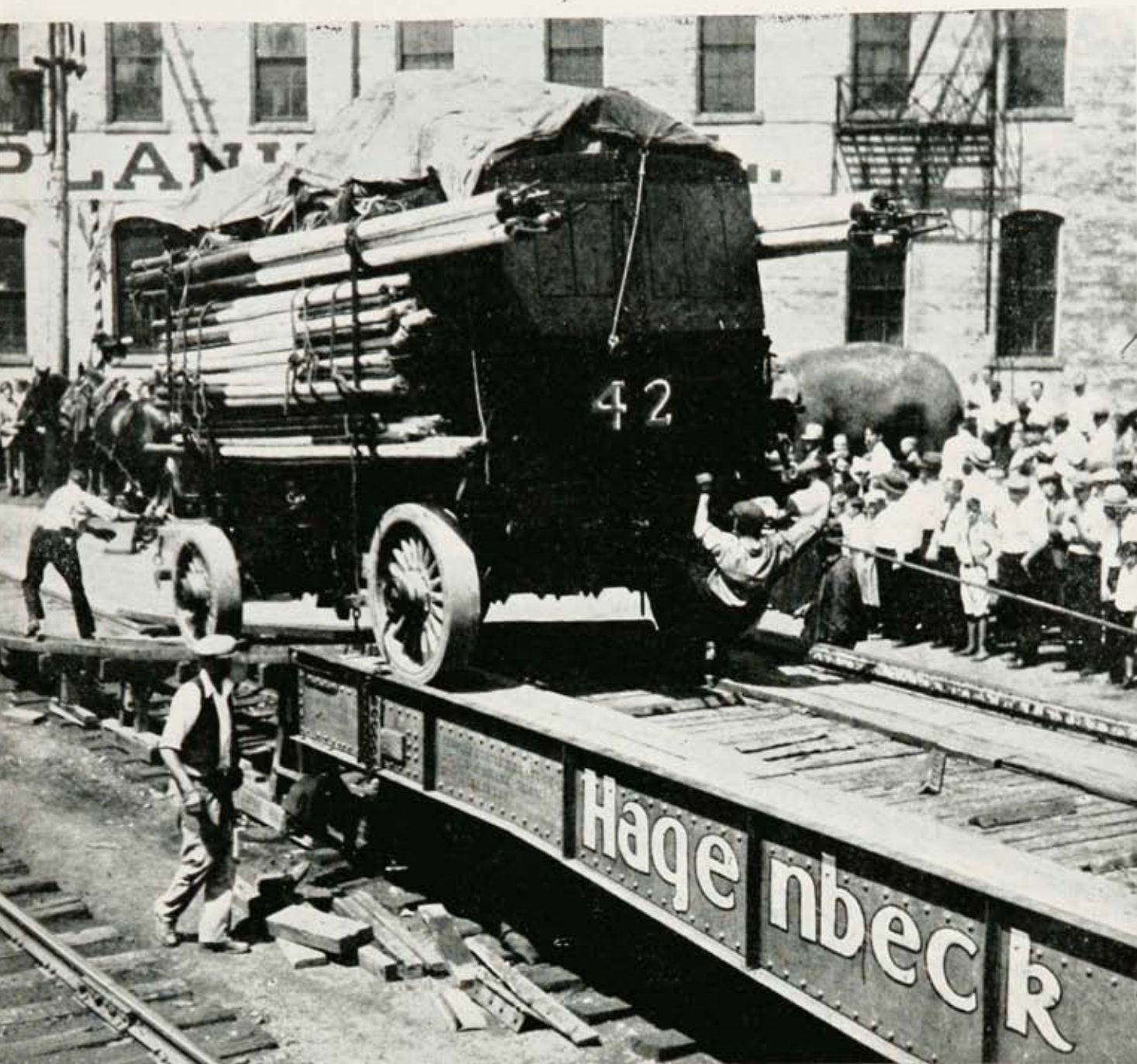
A loaded wagon comes off the flats and down the runs, with the "poler" shown in the dangerous job of guiding the wagon tongue or pole. Note the rope, which is attached to a snubber back on the car. Military men have studied circus technique of loading and unloading wagons on railway cars.
