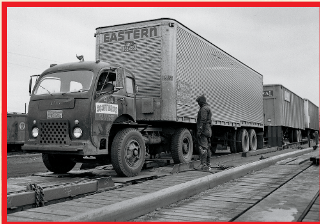
A car knocker checks the bridge plate ramp under a tractor trailer being unloaded "circus style" at the Pennsylvania Railroad yard in South Kearny, N.J., in January 1960. Don Wood
