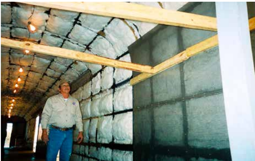
Here's the interior of a rebuilt generator car for the 2011 Red Unit circus train under rebuild at Ringling's Palmetto, Fla., shop with sound-baffling insulation. Rhett Coates
