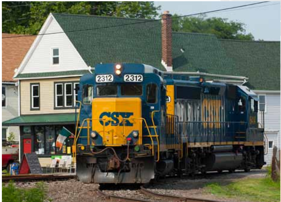
Its GP30 lines unspoiled, CSX road slug No. 2312 and GP40-2 mother 6414 pass McCarthy's pub in the First Ward section of Buffalo, N.Y.
